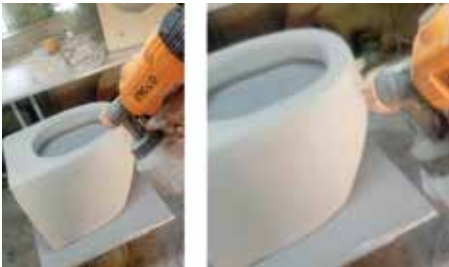
Spray glazing process
